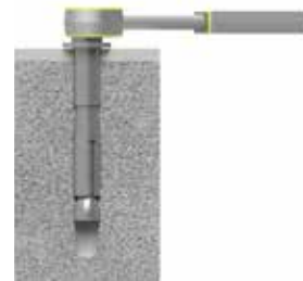
Tighten with torque wrench to Installation Torque
