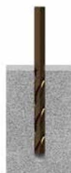
Position fixture and drill correct diameter hole to correct depth
