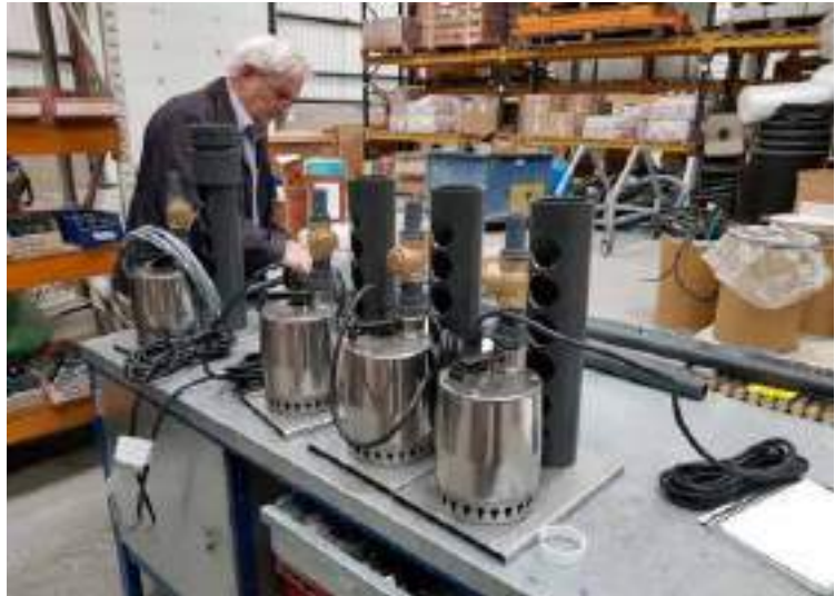
SPEL DrainGuard Bund Water Control Units supplied on this contract being inspected.
